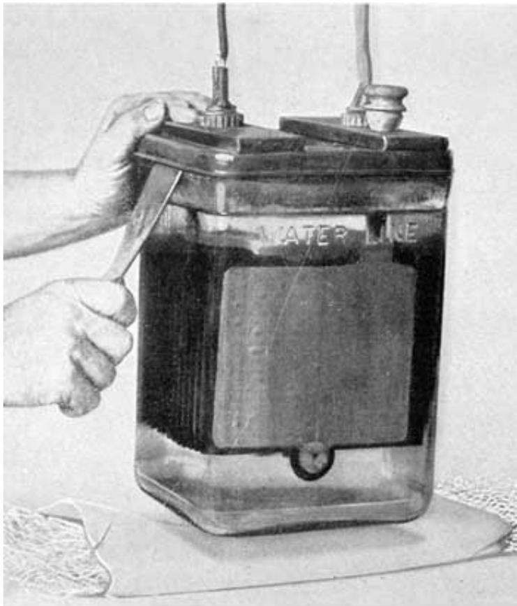
Fig. 306. Removing Delco-Light Cell Cover
