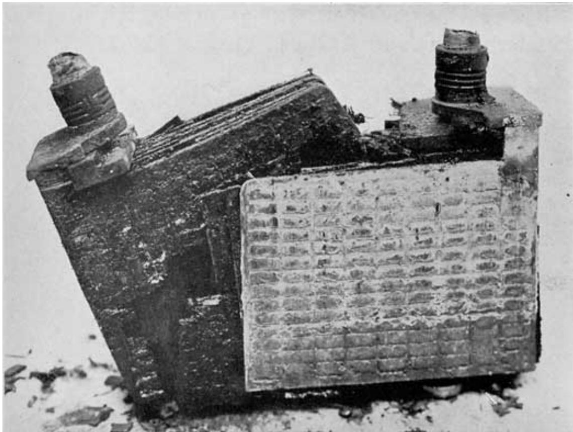
Fig. 209. Corroded, Bulged, and Sulphated Negatives.
