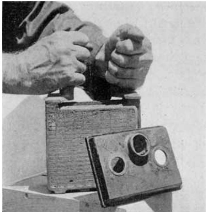
Fig. 227. Shifting Groups to Make Cover Fit
