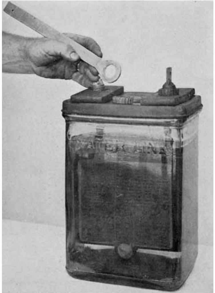
Fig. 320. Auxiliary Strap. Delco-Light Cell
