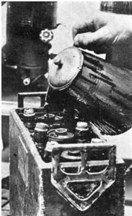
Fig. 229. Pouring Compound on Lower Covers
