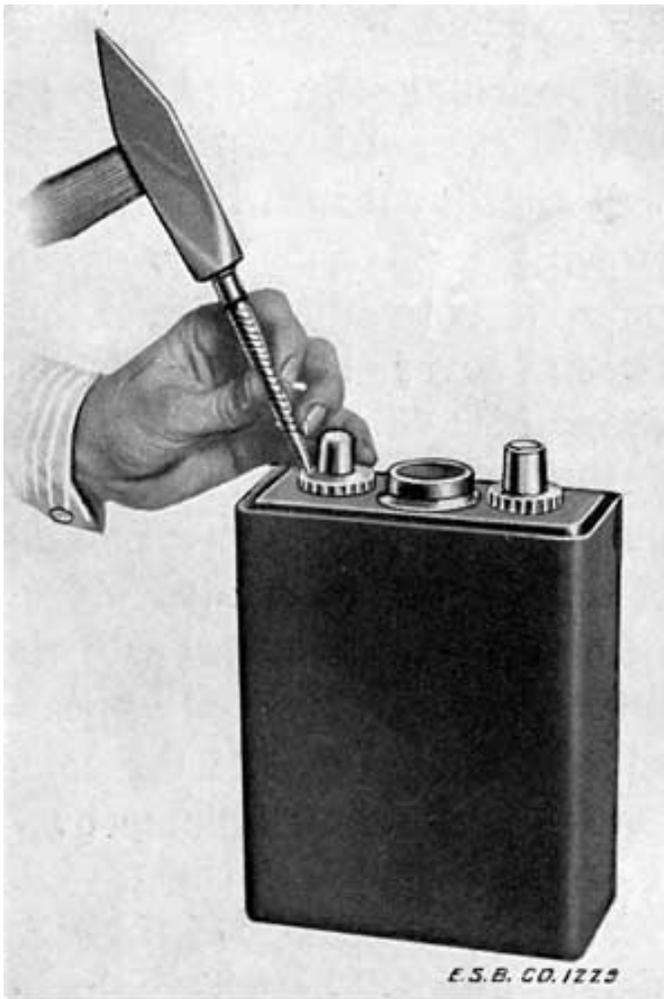
Fig. 241. Upsetting Threads to Prevent Nut from Turning
